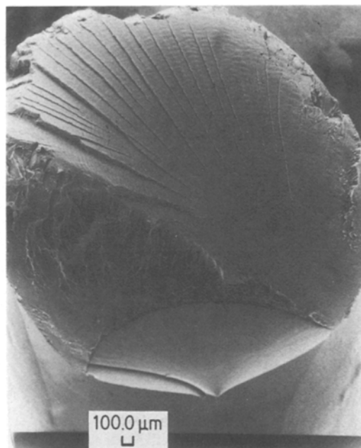
Figure 5 Fracture surface of uncoated HMW polymer; sample tested at 0.508 \text{ cm min}^{-1} .
