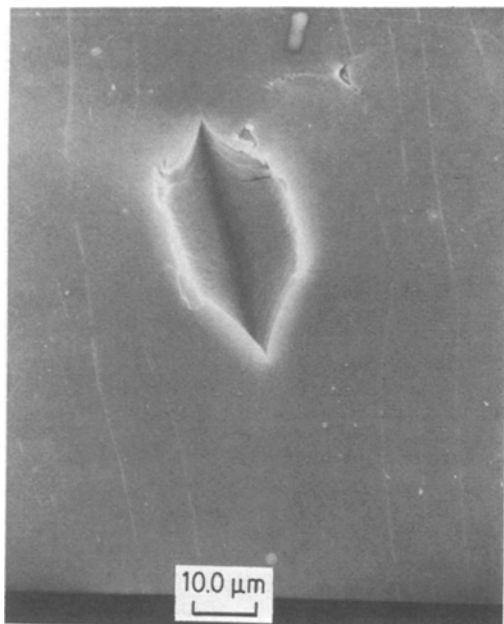
Figure 4 Free surface near to the fracture plane of uncoated HMW polymer; sample tested at 0.508 \text{ mm min}^{-1} .
